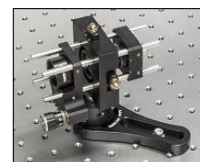
Click to Enlarge Figure 4: Spatial Filter System
